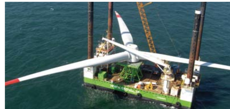
GeoSea's Vagant transporting a 126 m diameter wind turbine rotor to the Thorntonbank
